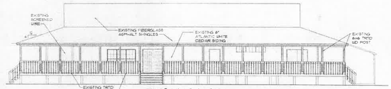
3 EX-1 SCALE: 1/8" = 1'-0" EXISTING NORTH ELEVATION
